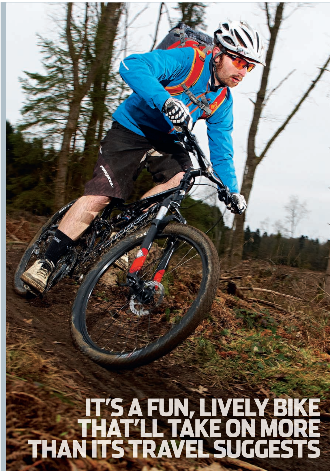
Steel-stanchioned Recon fork adds heft and lacks tunability, but does the job without fuss
