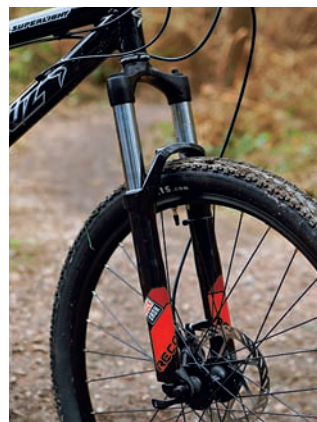
Steel-stanchioned Recon fork adds heft and lacks tunability, but does the job without fuss
