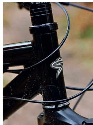
Conventional head tube with a standard 1.125in headset is a rarity these days
