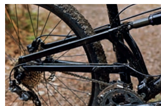
A pivot and a shock – and that's about it for the back end. Simplicity is a virtue
