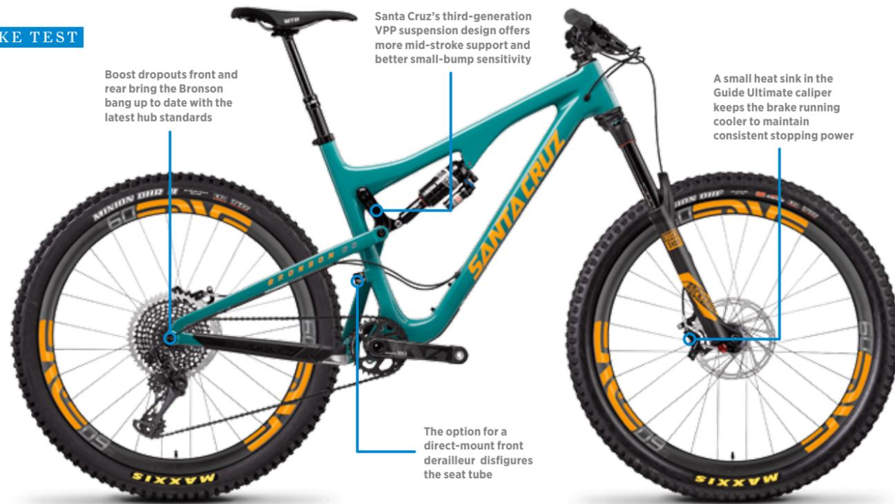
Boost dropouts front and rear bring the Bronson bang up to date with the latest hub standards
